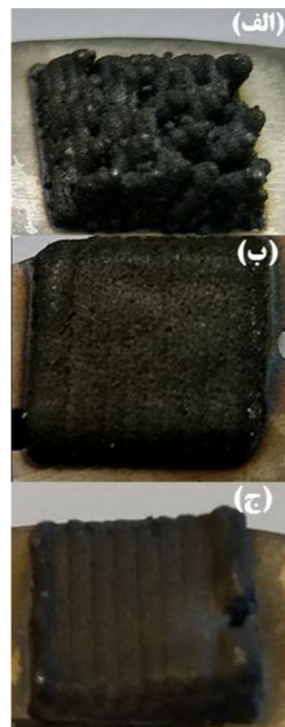
Fig. 7 Deposited samples with different power, A) 150 watts, B) 250 watts, C) 350 watts
