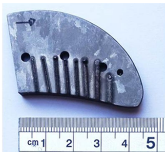
Fig. 3 Adjustment of LMD process parameters
