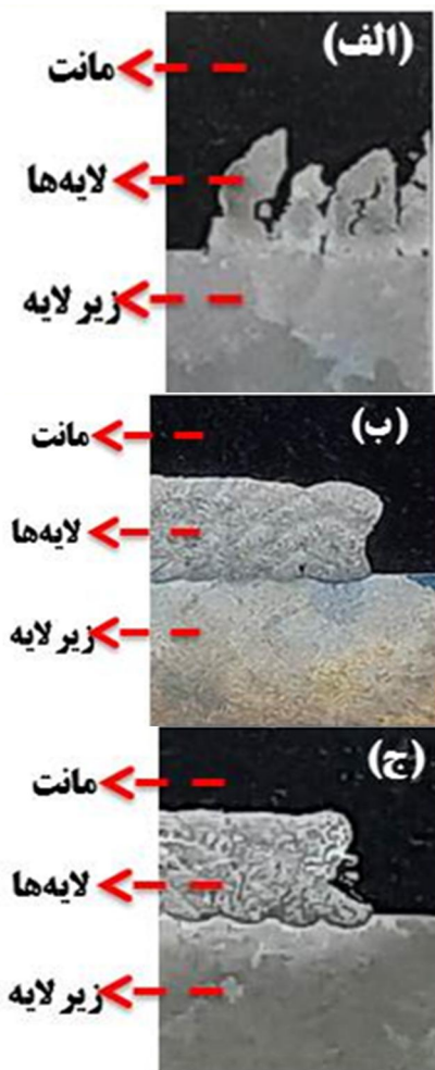
Fig. 8 A cross-sectional views of deposited samples with different power. A) 150 watts, B) 250 watts, C) 350 watts
