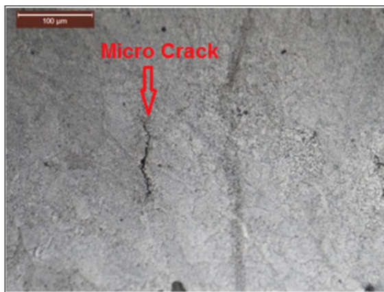
Fig. 11 The microstructure of IN625 Samples built SLM technique showing Micro Crack
