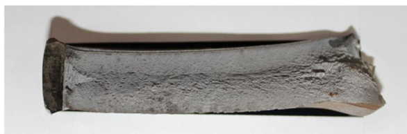
Fig. 4 The fracture surface of the drop weight tear test specimen with spiral welding
