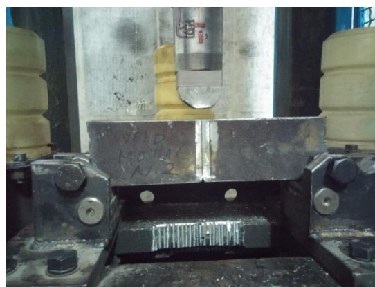
Fig. 2 Welded specimen in the drop weight tear test machine
