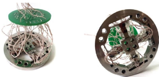
Fig. 10 Strain-gauges connection to the PCB
