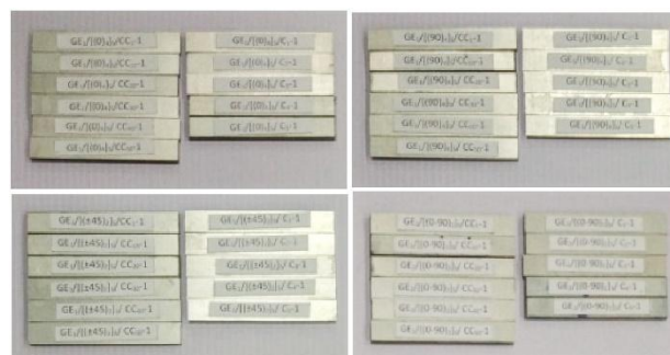
Fig. 3. The fabricated aluminium/glass fibers-epoxy FMLs
