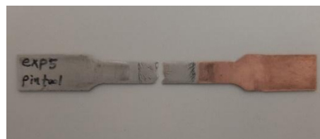
Fig. 5 Tensile test sample after failure
