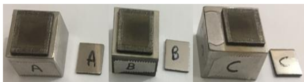
Fig. 8 Cutting the upper part of the samples using a wire cut machine
