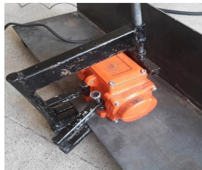
Fig. 3 Vibration stress relief setup on stress relief test
