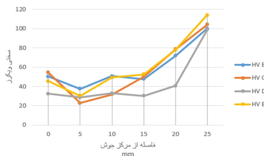
Fig. 10 Comparison of microstructure hardness of joints at different speeds B: 1500 rpm, C: 1180 rpm, D: 950 rpm, E: 750 rpm
