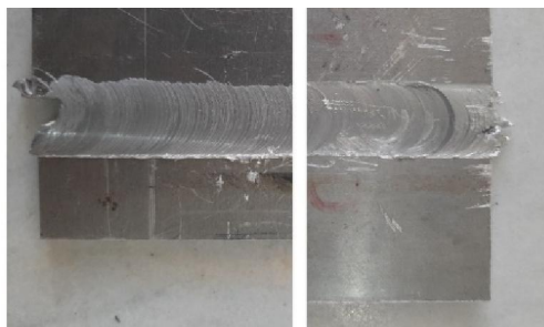
Fig. 8 Right: welding with a tool made of hot-worked steel and left: welding with HSS tool
