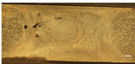
Fig. 22 Welding macrostructure performed at a speed of 1180 rpm with the help of Bobbin tool made from tool steel HSS
