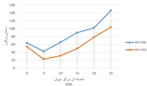
Fig. 13 Comparison of the hardness distribution in the microstructure of welded specimens at the same speed with the help of Bobbin tool made of H13 tool steel and hot-worked steel H13
