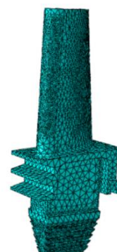
Fig. 8 Turbine blade mesh after study of mesh dependency
