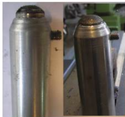
Fig 3 Spark machined magnet with its fixture
