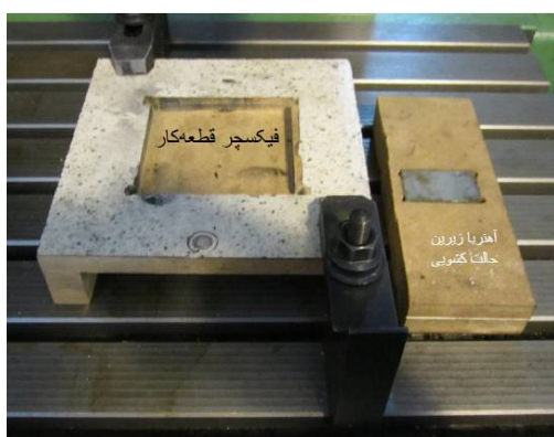
Fig. 4 Fixture for holding workpiece with magnets under the workpiece
