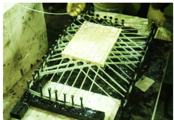
Fig. 7 Filament winding and fill grooves in silicone mold
