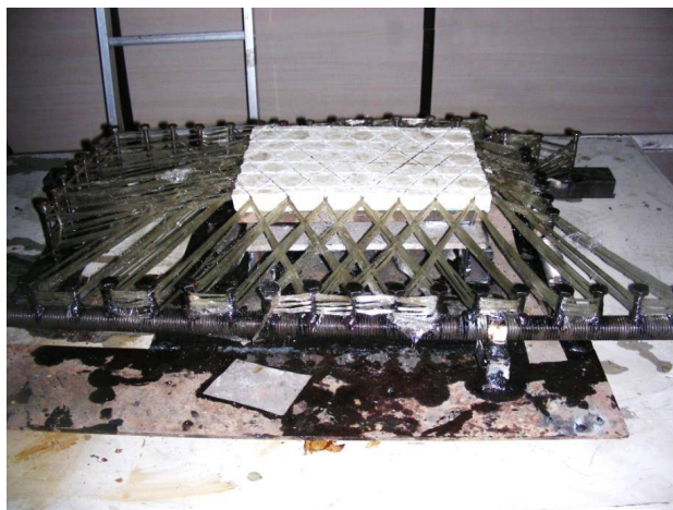
Fig. 9 Composite mesh panel threaded into a silicone mold after cure and before separation from the mold
