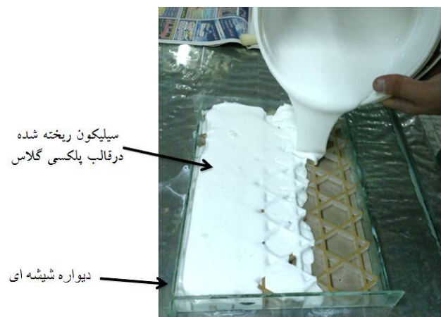
Fig. 4 Male mold located on a layer of Teflon surrounded by four glass walls
