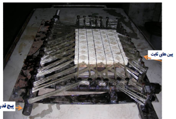
Fig. 11 Mechanism with fixed and movable screws located on the power screw
