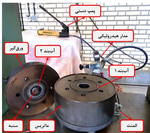
Fig. 2 A view of sheet hydroforming die set
