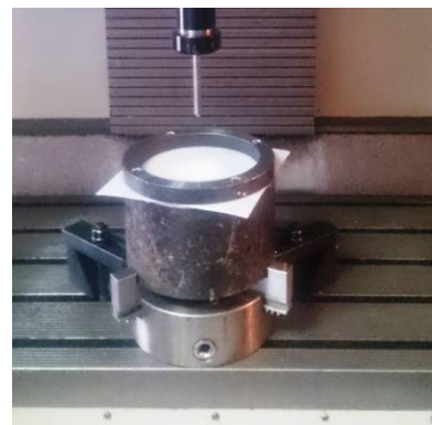
Fig. 15 The manufactured fixture to remove the curvature of produced parts
