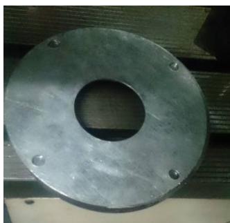
Fig. 5 The rigid support with the thickness of 2 mm
