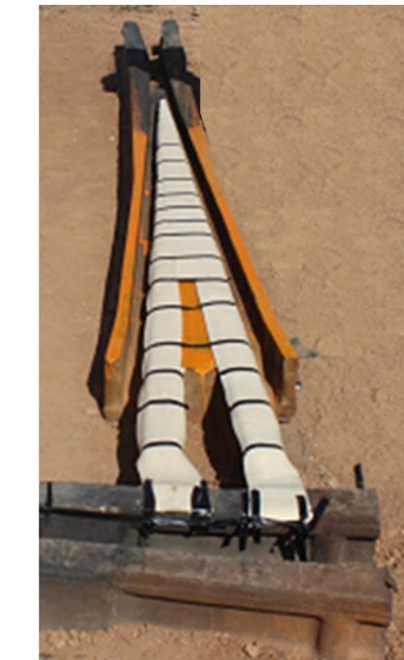
Fig. 16 The railway frog work-hardening process
