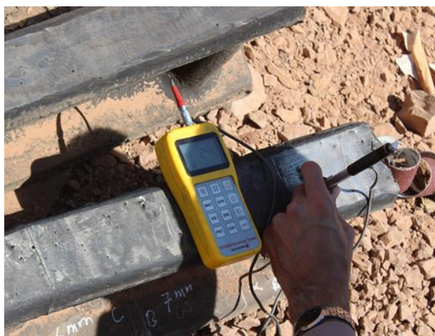
Fig. 13 Measuring the hardness of the specimens
