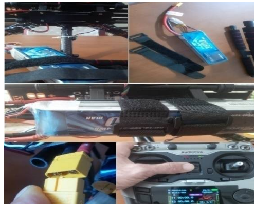
Fig. 12 Battery installation and radio control test
