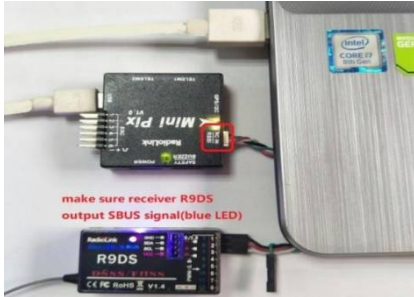
Fig. 14 Connection of the flight control to the computer for setting of the flight modes
