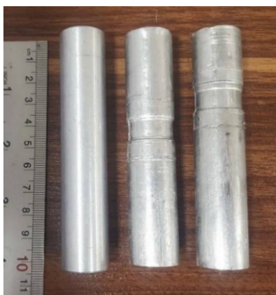
Fig. 4 The images of the tube from left to right related to before, during and after hydrostatic tube cyclic extrusion compression process, respectively
