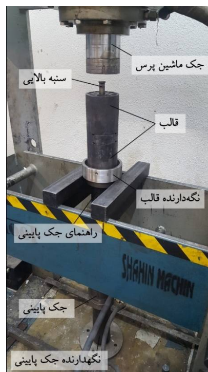
Fig. 3 The used setup for hydrostatic tube cyclic extrusion compression process
