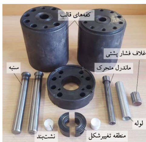
Fig. 2 The images of the die components of hydrostatic tube cyclic extrusion compression process
