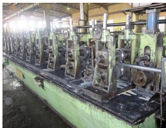
Fig. 7 The reshaping of folded cross section tube machine
