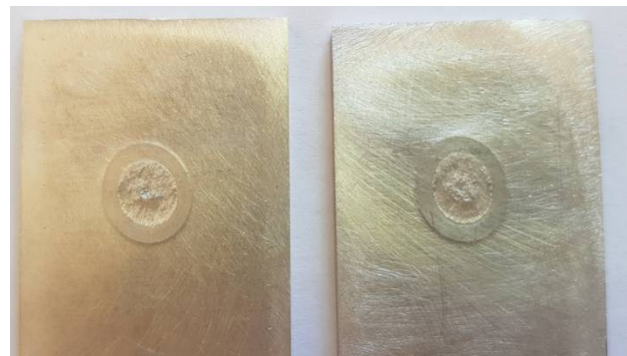
Fig. 7 The failure mode of spot welded joints
