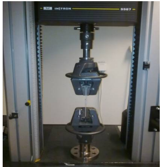
Fig. 2 The tensile-shear test of spot welded joint
