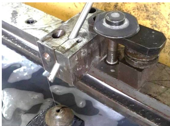
Fig. 6 Placing the pipe in the fixture when it cut with the wire-cut machine
