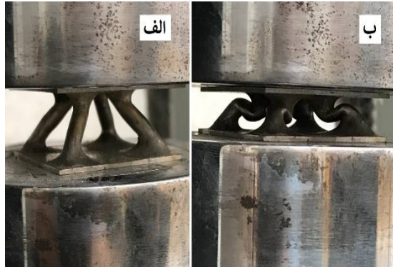
Fig. 13 Deformation of sample with L/d = 5 and w = 45 a) just before local buckling b) just before condensing
