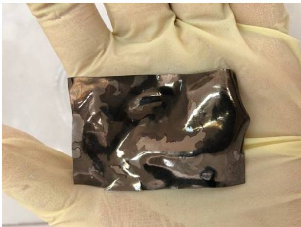
Fig. 5 Final manufactured ionic-polymer-metal composites
