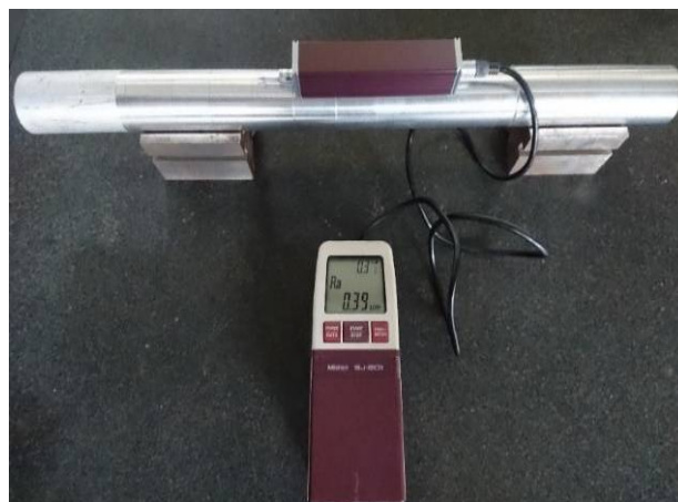
Fig. 4 Method of measuring surface roughness with measuring equipment
