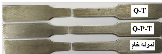
Fig. 5 Samples used after tensile testing.
