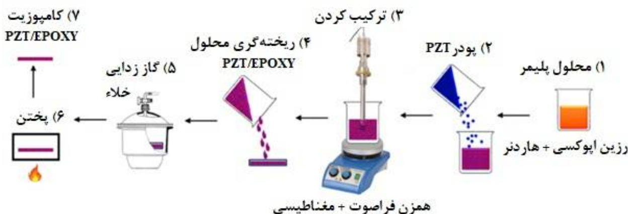
Fig. 4 Schematic representation of the steps involved in the present solution casting method
