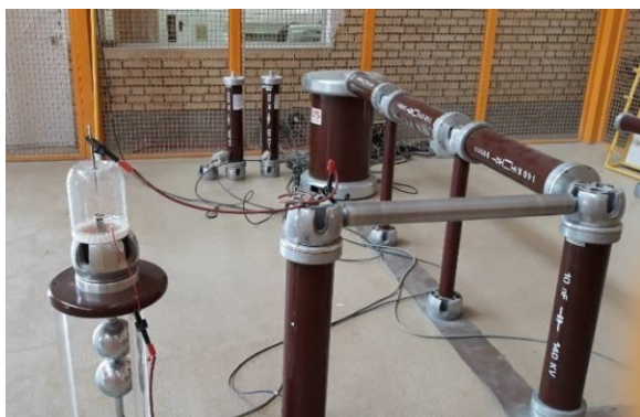
Fig. 7 The high-voltage setup for polarization of the samples
