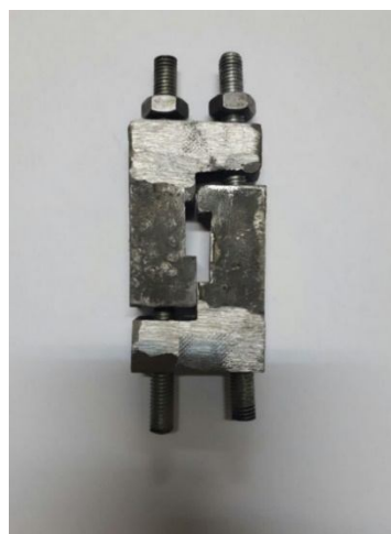
Fig. 3 The prepared fixture for shear strength test.
