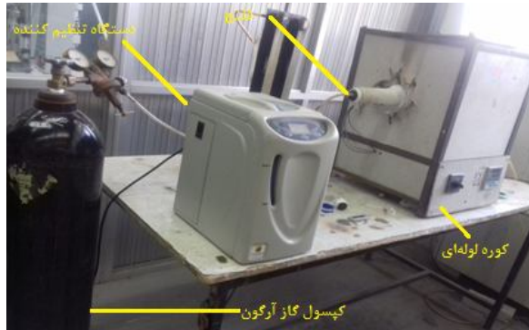
Fig. 2 The vacuum-furnace brazing process.
