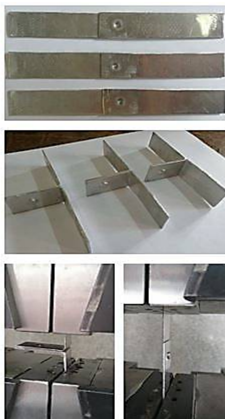
Fig. 14 Preparation of the clinched specimens to perform the shear and peel tests
