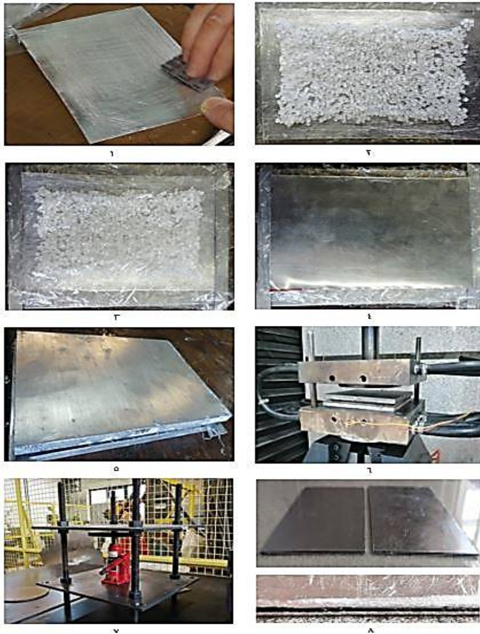
Fig. 7 Steps of preparing three-layer sheet
