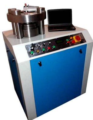
Fig. 10 General sheet testing machine model SMT-A 400 B
