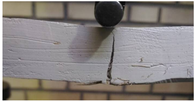
Fig. 5 Bridging mechanism after matrix cracking
