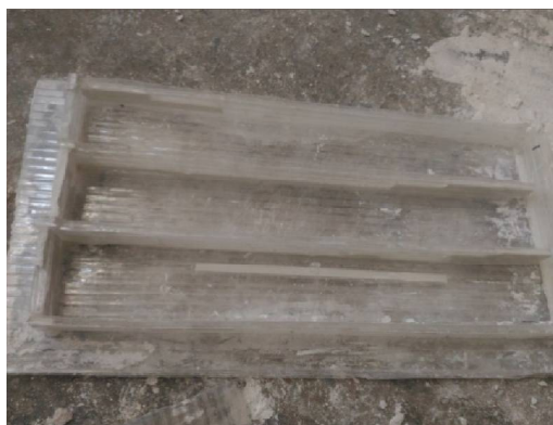
Fig. 1 Polycarbonate mold for producing composites
