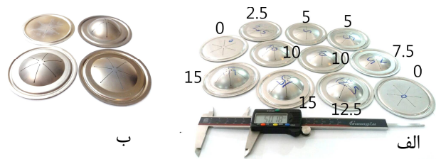
Fig. 4 a) Slotted bulge formed discs in different height b) annealed discs
