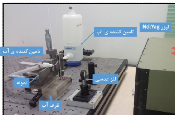
Fig. 3 LSP process setup
