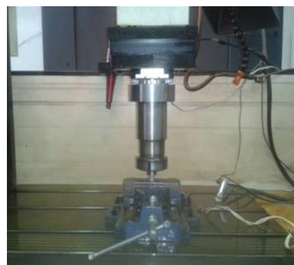
Fig. 1 Setting the electrode to electrical discharge process
