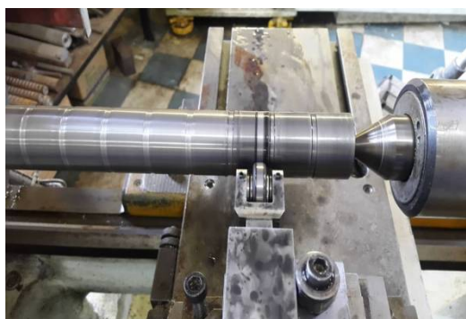
Fig. 3 Roller burnishing operation
