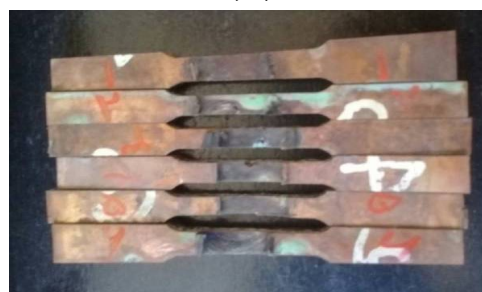
Fig. 4 a) Dimensions of tensile test samples, b) samples prepared for tensile test
