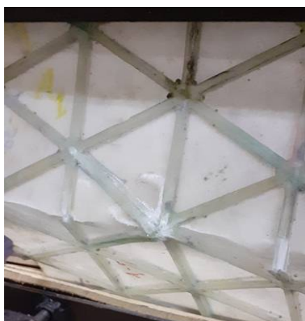
Fig. 5 Failure of impacted plate under compression loading
