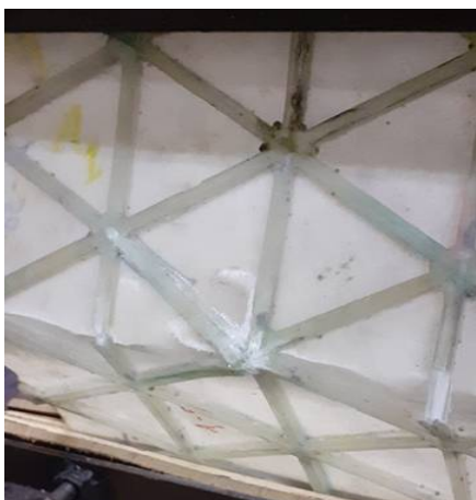
Fig. 5 Failure of impacted plate under compression loading
