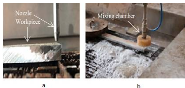
Fig. 2 Cutting sample using abrasive water jet machining. (a) SOD setting; (b) Operation of material cutting
