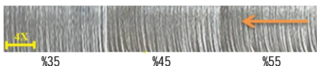
Fig. 20 image of impact of loading factor change on angle of striation (jet pressure 280 MPa, traverse speed 200 mm/min)
