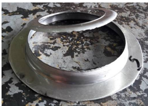
Fig. 8 Tearing of flange wall because of small initial hole diameter
