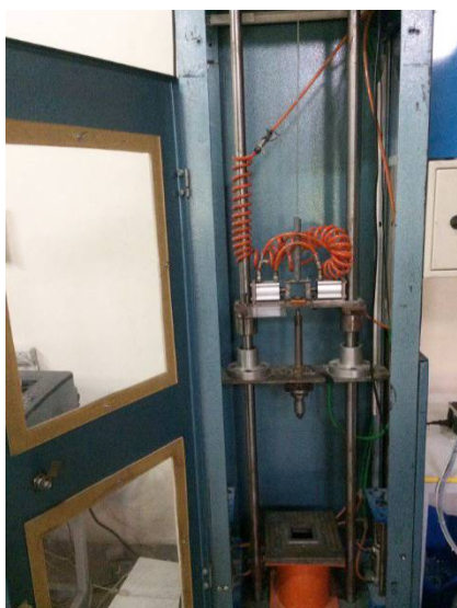
Fig. 2 Drop-weight Low Velocity impact test device
