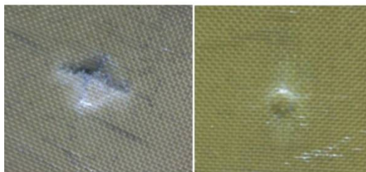
Fig. 6 View of front and behind of sample 1 (K13) after impact test
