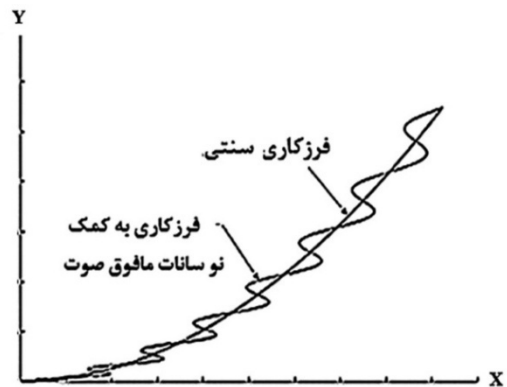
Fig. 4 The tool moves in traditional milling and ultrasonic assisted milling
