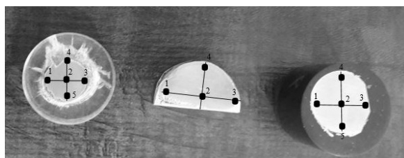
Fig. 10 Cross-sectional sample with specified points for hardness measurement a) sample after pass two b) first pass sample after forging c) sample after pass one
