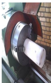
Fig. 1 Schematic and actual views of centrifugal method to make a FGM
