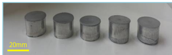
Fig. 4 Fabricated samples by dynamic compaction method
