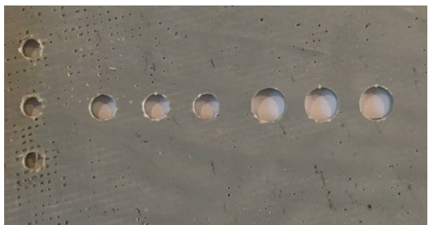
Fig. 5 Drilling of GFRP composite plate
