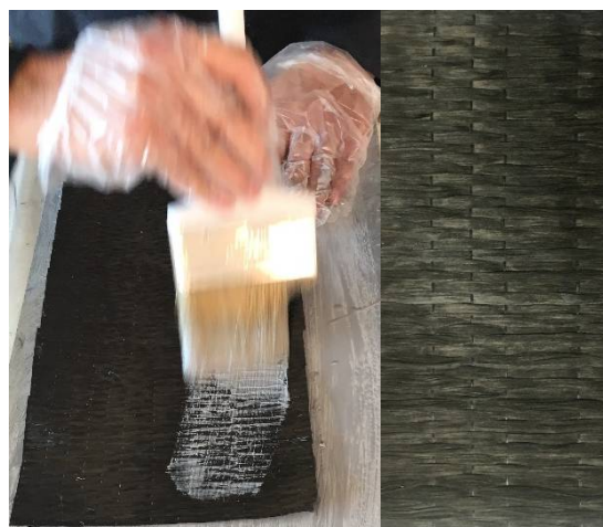
Fig. 2 Hand layup for manufacturing CFRP
