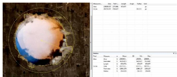
Fig. 10 Image processing for 2 mm CFRP with 10mm drilling diameter and a feed rate of 200 mm/min
