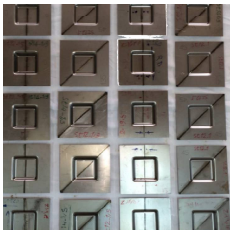
Fig. 10 Samples of parts formed in the form of a truncated pyramid in SPIF at two sides of the weld line.
