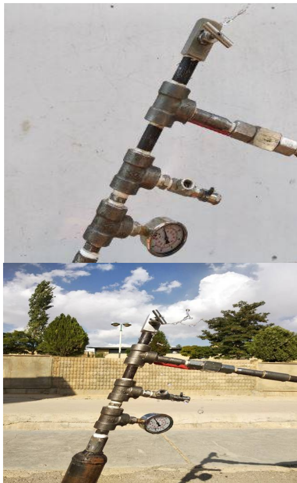
Fig. 5 Bleeding an experimental specimen
