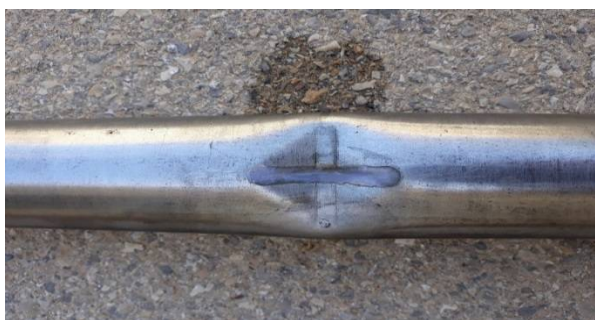
Fig. 7 An experimental repaired specimen after the indentation test
