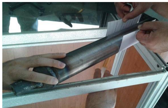
Fig. 2 Repair trend of the damaged tube by the resin
