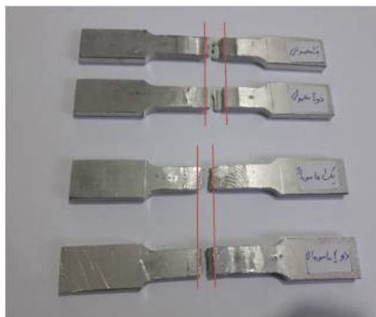
Fig. 8 The fractured samples under the tensile test
