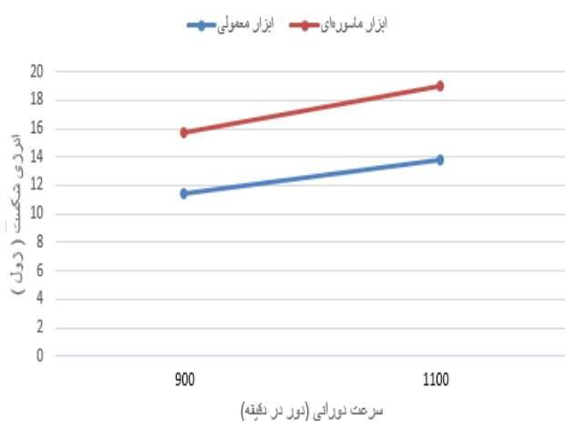
Fig. 9 The effect of the rotational speed on the failure energy
