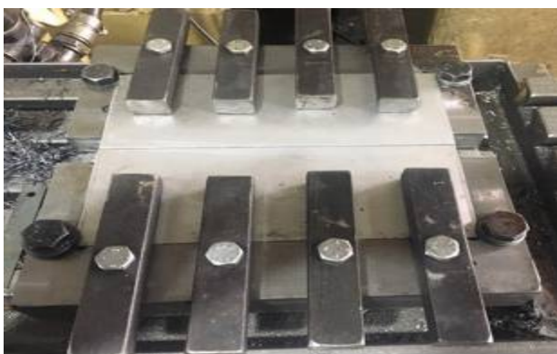
Fig. 3 The welding samples in the fixture
