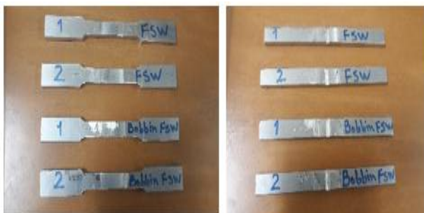
Fig. 4 The prepared samples for the tensile and Charpy impact tests
