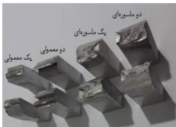
Fig. 10 The fractured samples under the Charpy impact test
