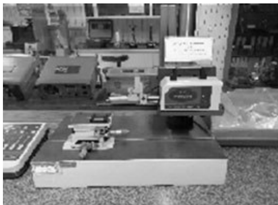
Fig. 5 Experimentally determined Surface roughness of AZ61 sheets with Ra value of 1.2 \mu\text{m}
