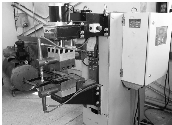
Fig. 2 Novin Sazan spot welding machine
