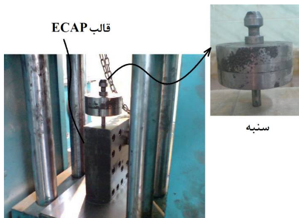
Fig. 3 Picture of die and punch in this study
