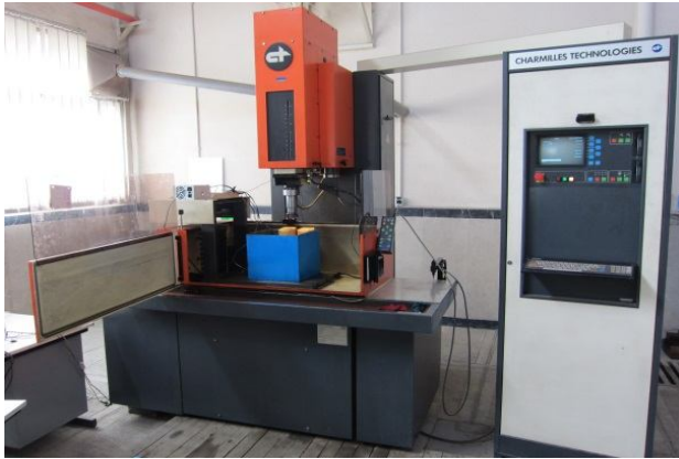
Fig. 1 The used CNC-EDM machine and the special powder mixing tank in the main tank of EDM machine
