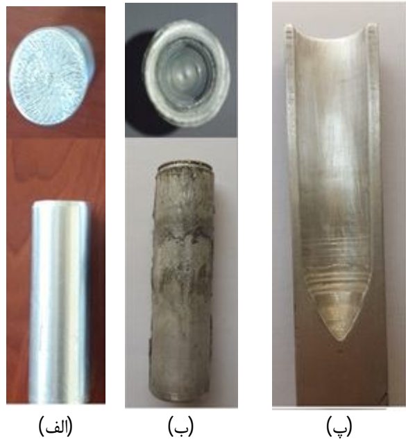
Fig. 3 illustrations of; (a) the initial specimen, (b) the final processed tube, (c) cross-section of the formed tube
