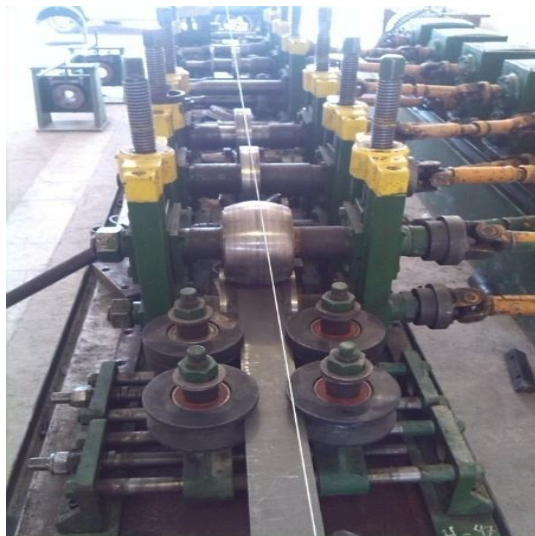
Fig. 6 Cold roll forming machine used in experiments
